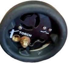
If you manage to overheat the high-voltage coil (by prolonged continuous fire) the Pig will shut down and sing. This is not dangerous or damaging, just annoying.
